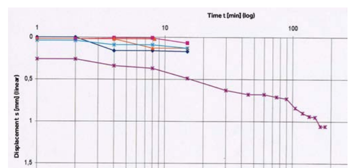
Suitability test: Determination of creep values
