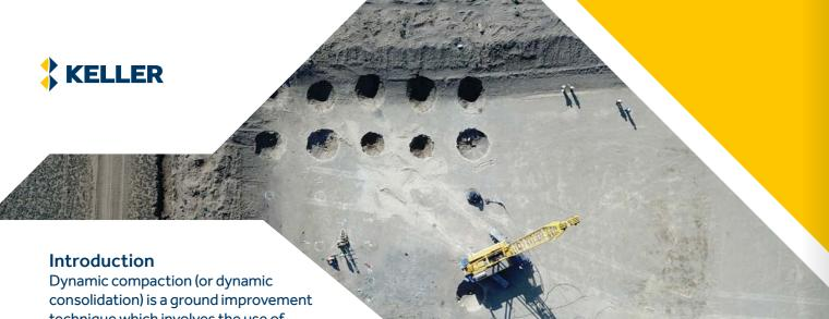
consolidation) is a ground improvement technique which involves the use of freefalling weights (or pounders) to improve the density, bearing capacity, stiffness and
